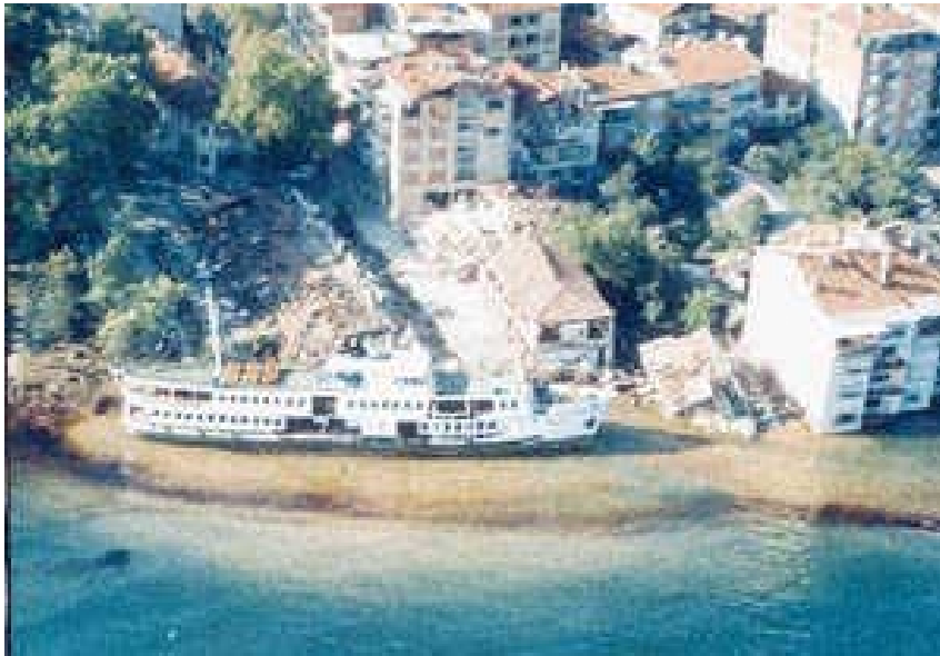
Figure 11.2 A passenger ship at De ĭrmendere where a submarine landslide took place
