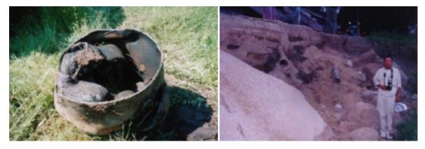
Figure 8.2 Buckling of water supply steel pipe
