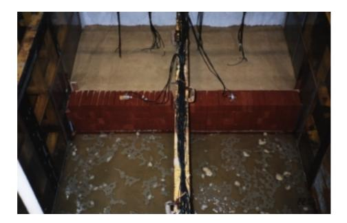
Figure 6.10 Underwater shake table test models
